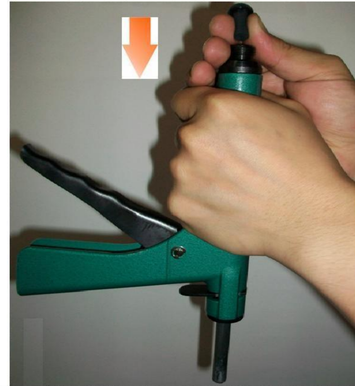
4. Set mushroom plug into Plugger with stem down
