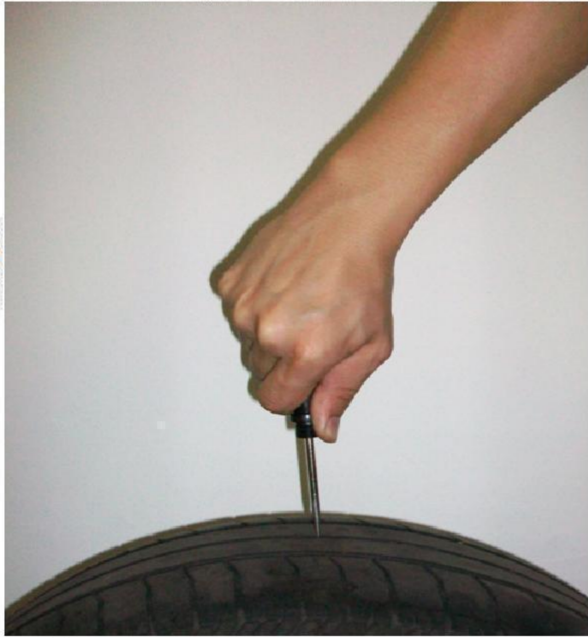
1. Use probe tool to inspect damage
