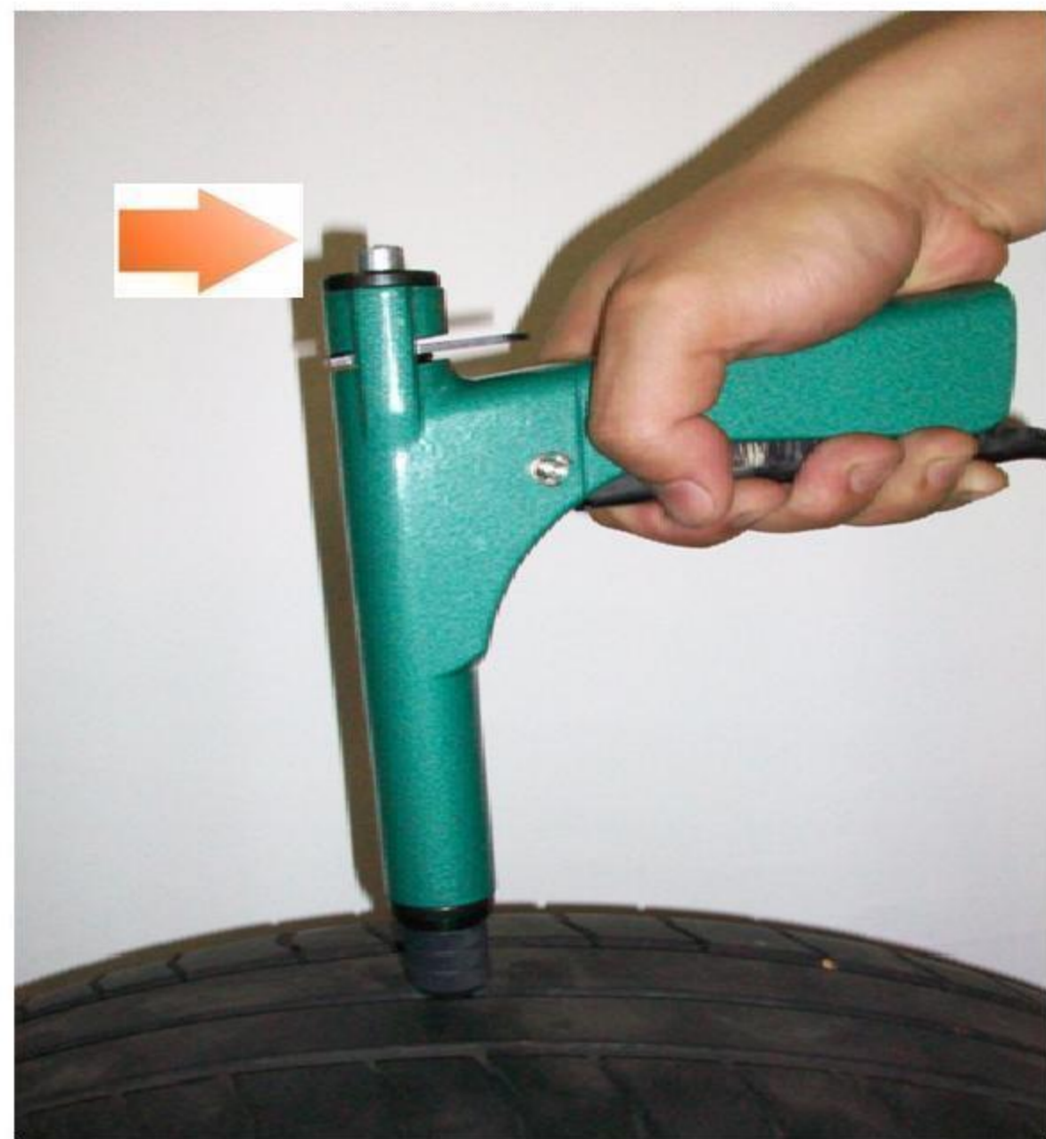
10. Push rod will force the plug into the puncture
